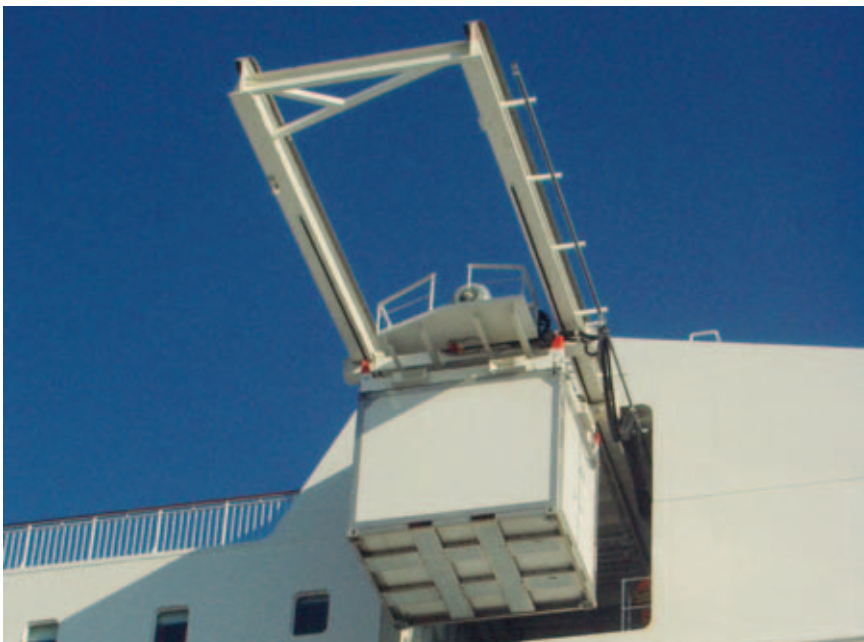
Container Crane SWL 7.5t Class BV Outreach 8.0m
