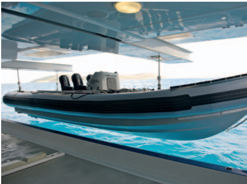
Electric Tender Boat Crane SWL Fwd 2 x 2.5t / Aft 4 x 2.0t Outreach 3950mm over both ship sides Class LR
