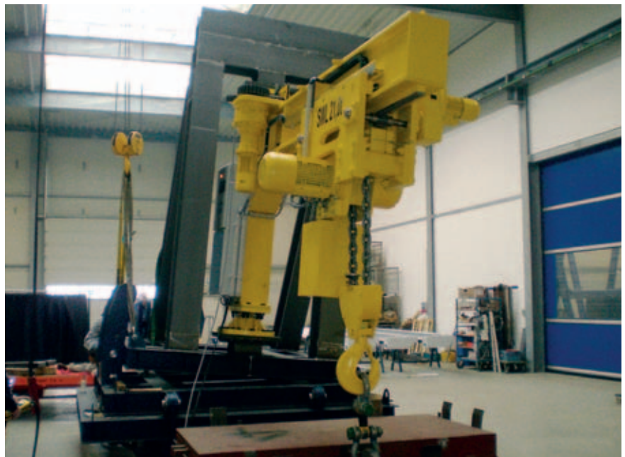
Slewing Jib Crane SWL 21t Outreach 3675 mm Class BV
