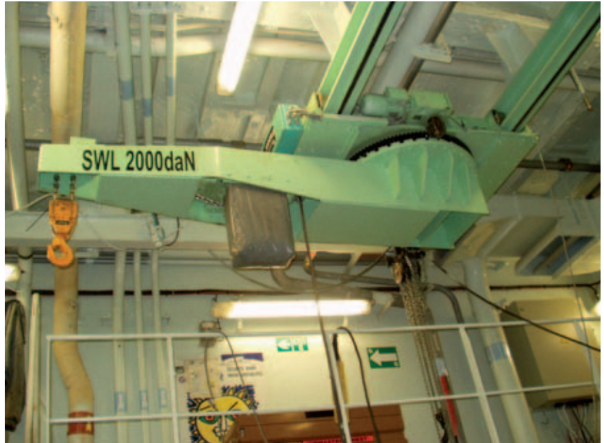
Slewing Jib Crane SWL 2.0t Class DNV
