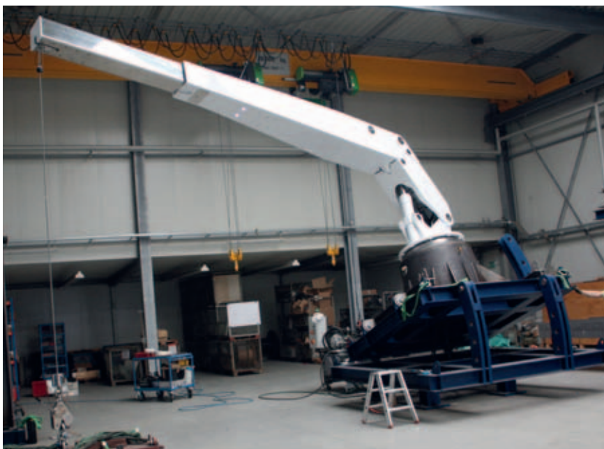
Hydraulic Rescue Boat Crane SWL 2.0t Outreach 6500mm Class GL/LR
