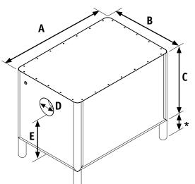
Above ground separator has a smooth cover plate and is supplied with height adjustable feet which increase dimension 'C' by 100 - 125mm.
